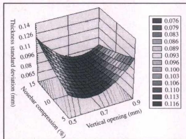
Fig. 2: Veneer thickness standard deviation response surface graph in the function of nosebar compression and vertical opening with clearance angle fixed at 1°
