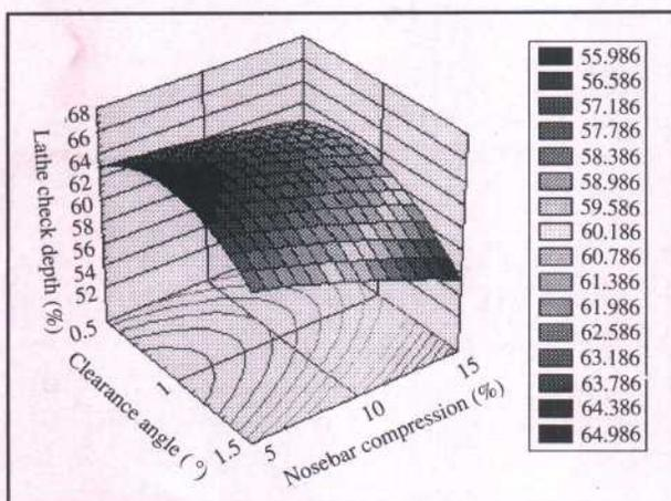
Fig. 5: Lathe-check depth response surface graph in the function of nosebar compression and knife clearance angle with vertical opening fixed at 0.7mm
