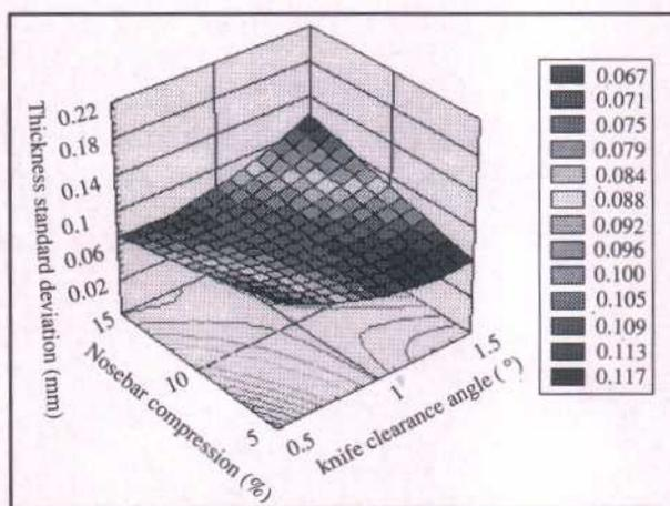
Fig. 3: Veneer thickness standard deviation response surface graph in the function of nosebar compression and clearance angle with vertical opening fixed at 0.7mm
