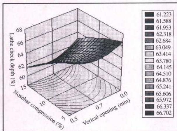
Fig. 4: Lathe-check depth response surface graph in the function of nosebar compression and vertical opening with knife clearance angle fixed at  $1^\circ$
