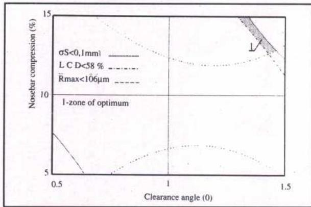
Fig. 7: Superimposed response contours of veneer thickness standard deviation, veneer roughness and lathe check depth, in function of nosebar compression and knife clearance angle
