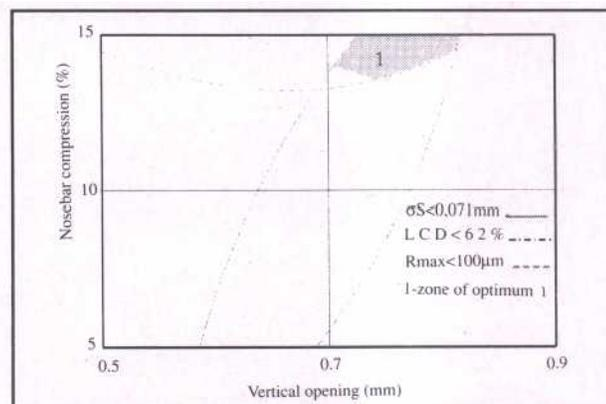
Fig. 6: Superimposed response contours of veneer thickness standard deviation, veneer roughness and lathe check depth, in function of nosebar compression and vertical opening
