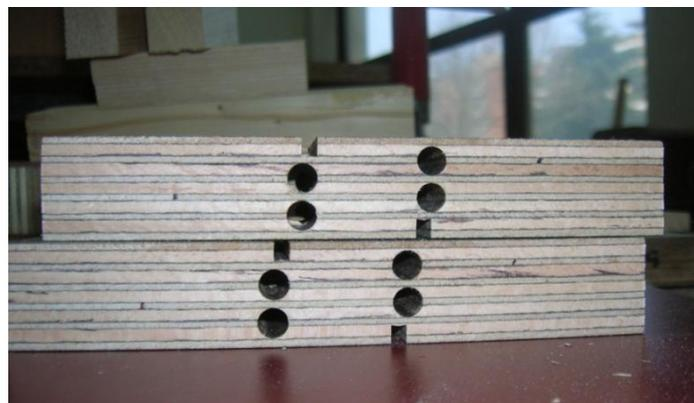
**Figure 1.** The look of the testing probe according D.A8.067
