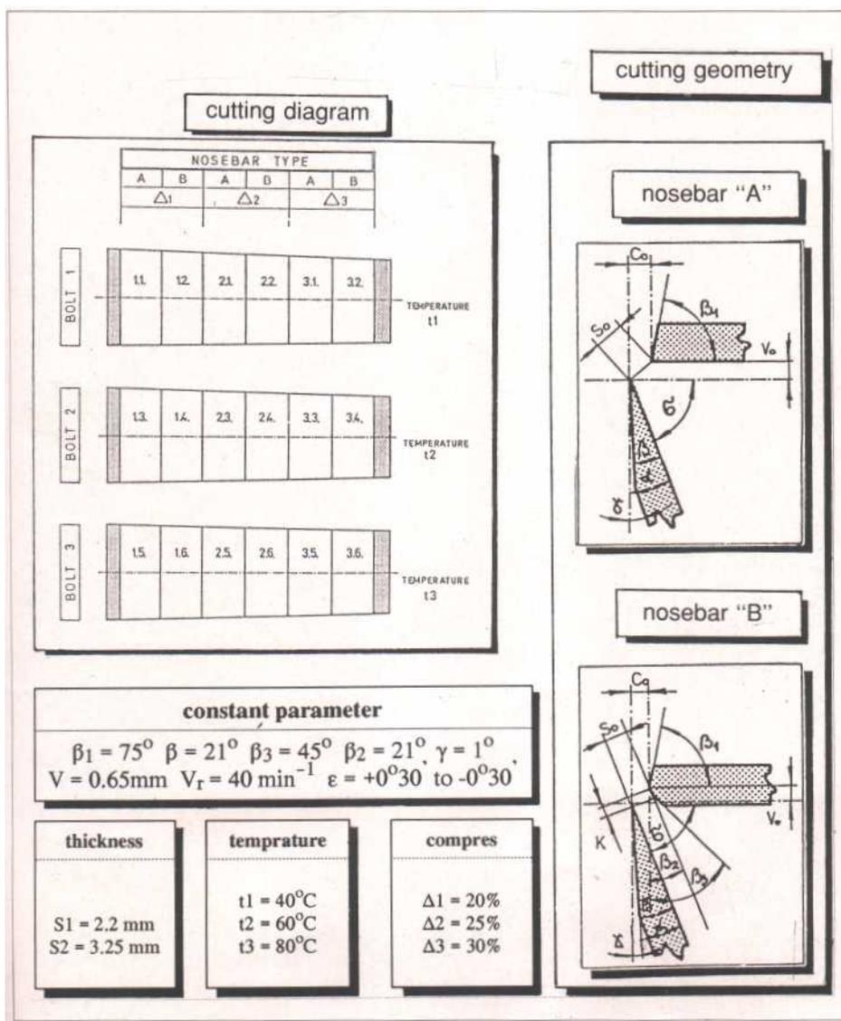
Fig. 1. Cutting diagram and cutting geometry
