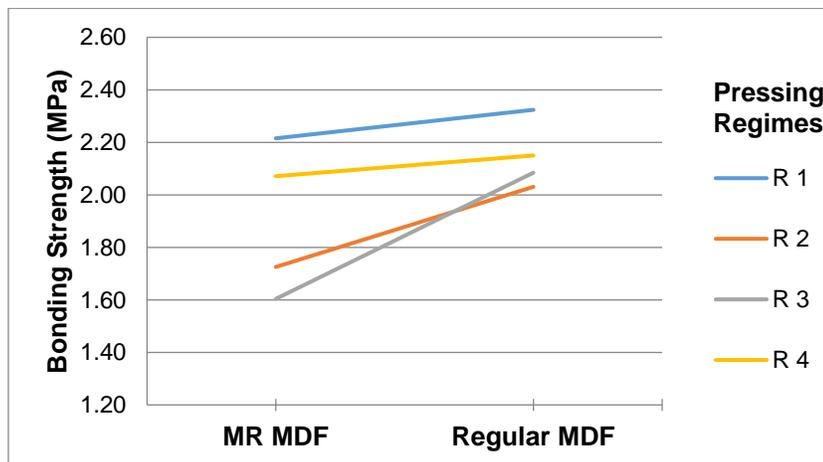
Fig. 6. Influence of substrate type and pressing regime on the bonding strength of oak veneer
