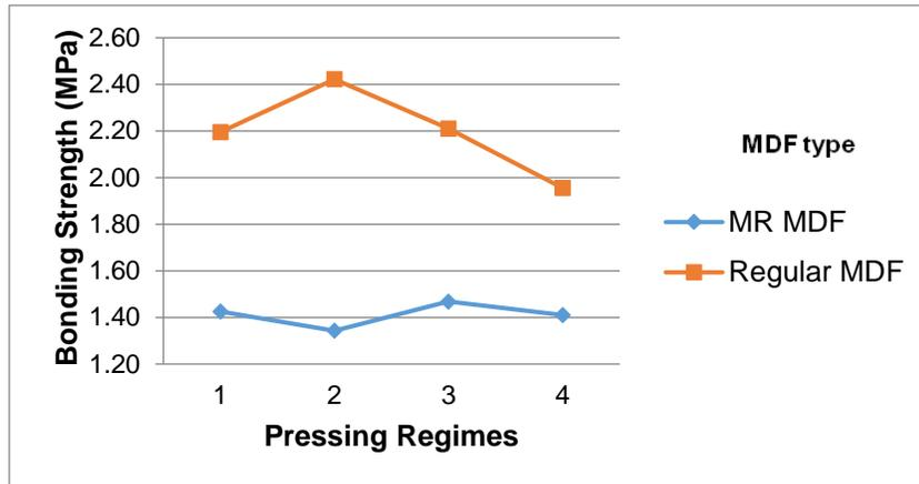
**Fig. 8.** Influence of substrate type and pressing regime on the bonding strength of beech veneer
