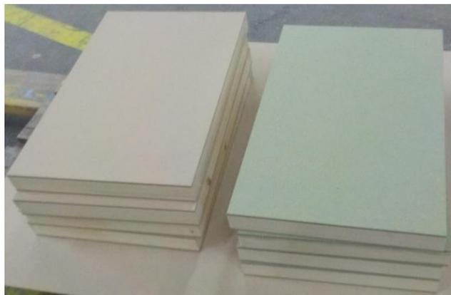
**Fig. 2.** Small-scale door construction from regular MDF (left) and moisture-resistant MDF (right)
