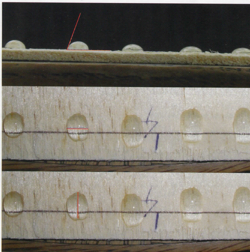
Figure 1: Method of measuring the contact angle ( \theta ) and spreading area in (x) and (y) direction
