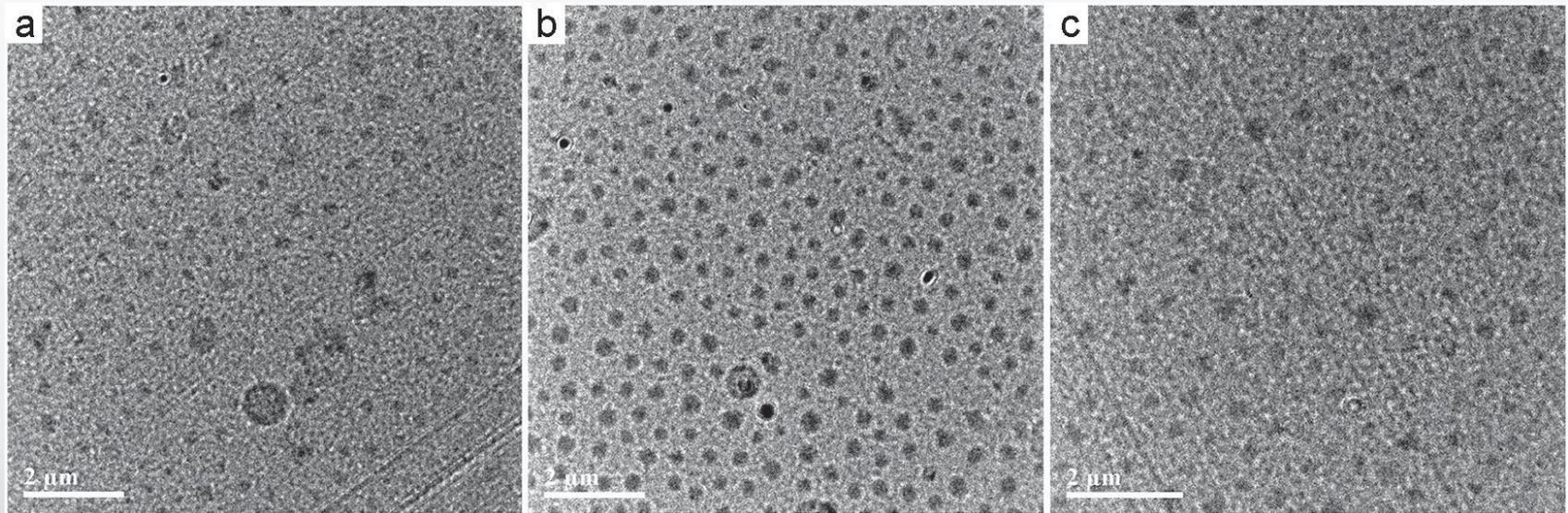
TEM images of lignin epoxy composites with 0.5%, 1.0%, and 1.8% of de-lignin–epoxide loadings a-c) after ultracut by microtome.
